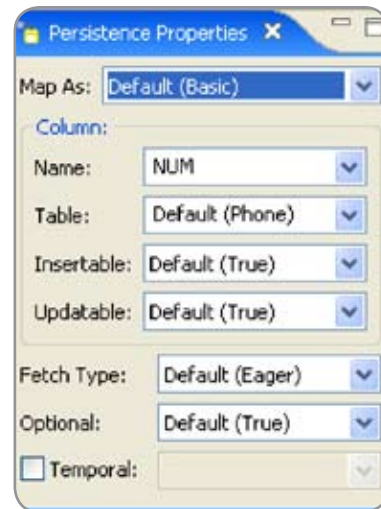
Figure 5 The Persistence Properties View displays the settings for mappings explicitly defined by the developer and the defaults that are implicitly applied by JPA runtimes
