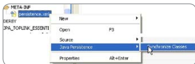
Figure 10 The list of Entities can be updated in the persistence.xml using the 'Synchronize Classes' menu option
